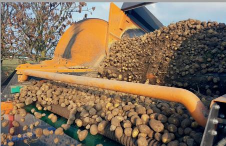
**Perfect cleaning:** The crop is nicely spread on the cleaning rollers thanks to the steady supply of crops by the discharge floor of the overload trailer.
