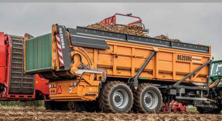
**Optimal loading space:** As the TC also functions as a folding rear tailgate, there is no additional rear overhang.
