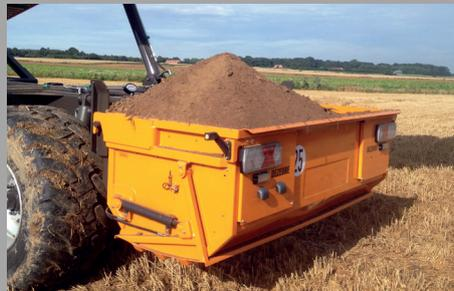
**No dirt on the road:** The soil is collected in the hydraulically operated soil-collector and can be unloaded evenly at a suitable location in the field.
