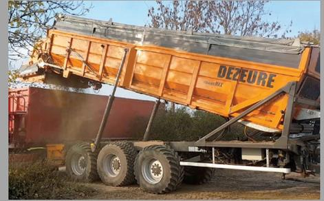
**Unloading, anywhere at any time:** The overload trailer unloads from the back, trailers can be loaded anywhere in the field.
