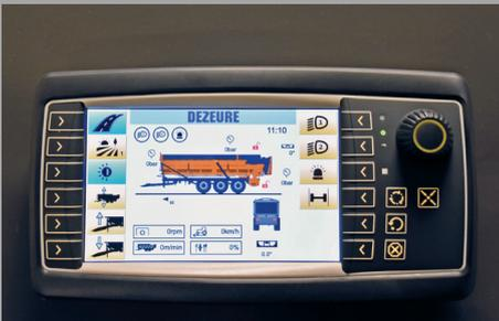
**Safe and easy:** Due to the **SecuTouch** touch-screen terminal, the TC is safe and easy to use. The SecuTouch terminal will automatically stabilize and level the trailer before operation.
