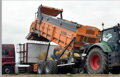
**Turbo output:** With a cleaning surface of +/- 5m<sup>2</sup>, the TC can ensure both cleaning of the crop and loading lorries in short time. Less than 10 minutes are required to load a full lorry.
